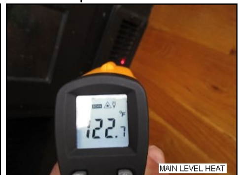
Heat tested functional - Adequate temperatures noted
